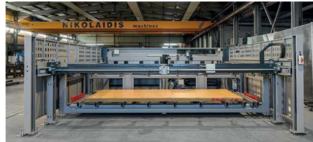
Heavy Duty lifting table platform: In standalone frame to avoid vibrations on machine's stability. Moving on 4 large trapezoidal screws. Maximum lifting capacity 600mm.
