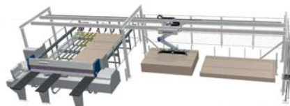
Automated magazine – panel storage system
