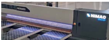
Blinking White Light Indicated precise panel positioning - Error-free system
